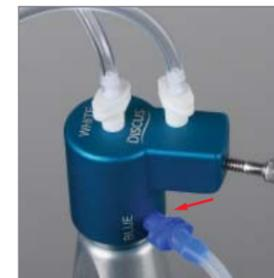
**Figure 5.** Firmly insert the opposite end of the MDT tubing set (blue connectors) to the lower port of the Multi-Port Adapter (red arrow).
