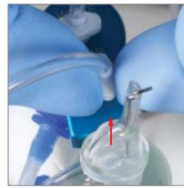
**Figure 12.** Remove the white connector closest to the front of the Multi-Port Adapter (red arrow).
