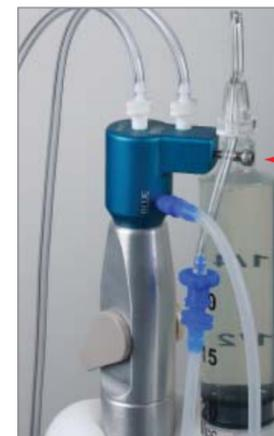
**Figure 6.** Hang the MDT on the screw (red arrow) attached to the front of the Multi-Port Adapter.
