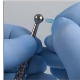
**Figure 11.** Firmly insert the MacroCannula into the Handpiece.
